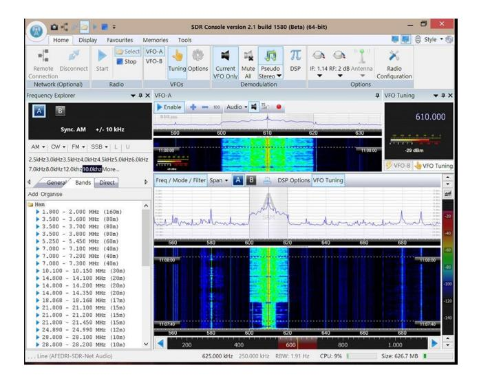
The controls are all laid out nicely in SDR-Radio V2.1 and the user can expose band, filters, and recording controls and a full spectrum view on an as needed or permanent basis. In this view I am set to a simple local AM station using a Wellbrook Loop. Audio is exceptional at 10K width!
