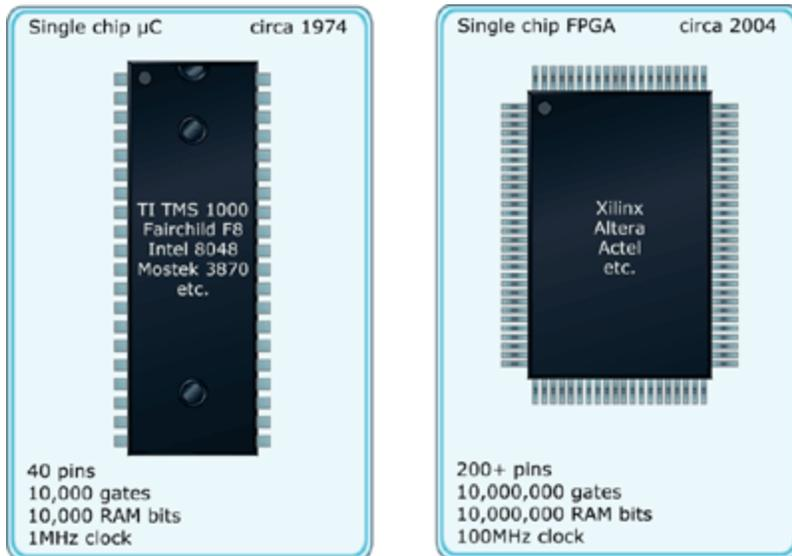
**Figure 1: Comparison of first microprocessors to current FPGAs**
