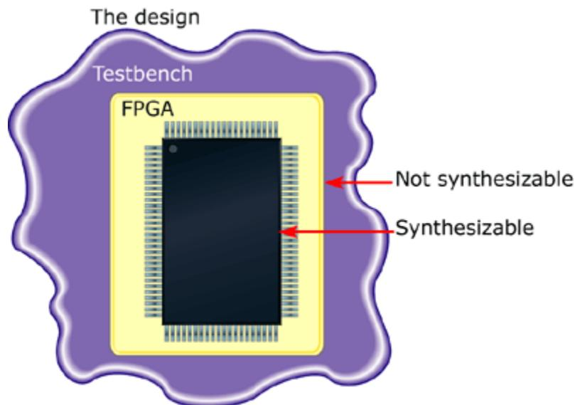
**Figure 2: Synthesizable and nonsynthesizable portions of design**
