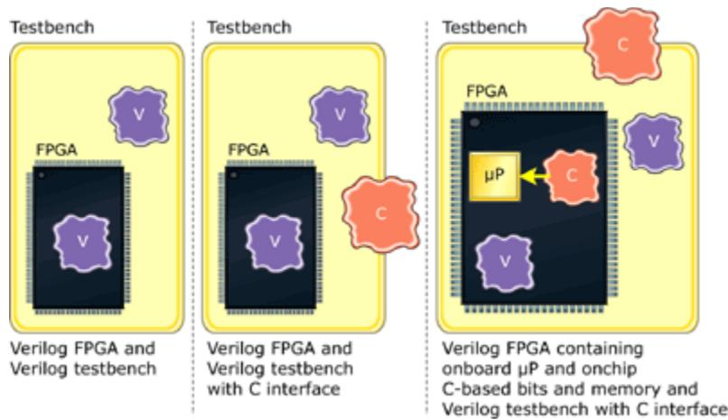
**Figure 3: Testbenches and C code in debugging**
