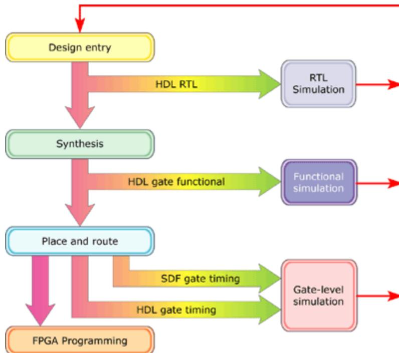
**Figure 4: The FPGA programming process**
